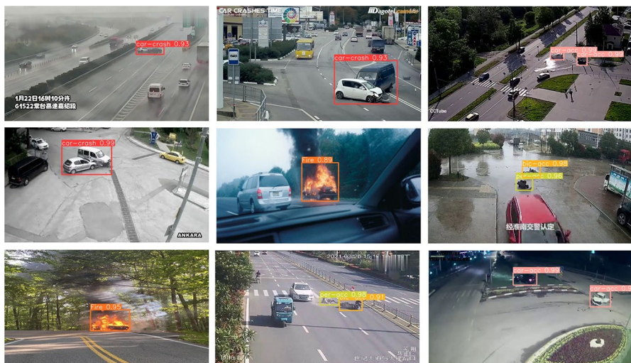
Fig. 16 Test results of TP-YOLOv8n model using TAT dataset on NVIDIA Jetson TX2 NX platform
