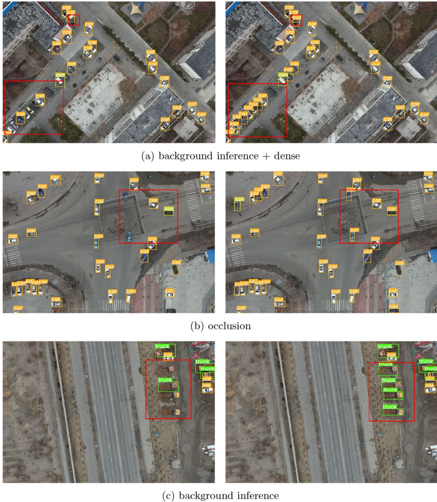
Fig. 16 Comparison of the detection performance of YOLOv8n and LightUAV-YOLO in a variety of different scenarios captured by the drone. The left column presents the results from YOLOv8n, while the right column displays the detection results from LightUAV-YOLO. The red bounding box shows more obvious contrast situation
